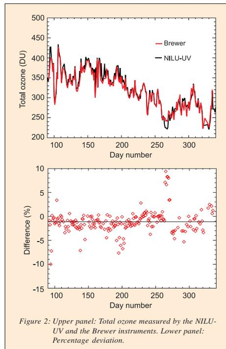
Figure 2: Upper panel: Total ozone measured by the NILU-UV and the Brewer instruments. Lower panel: Percentage deviation.
