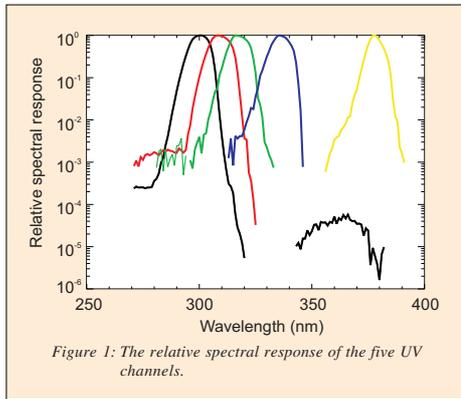
Figure 1: The relative spectral response of the five UV channels.
