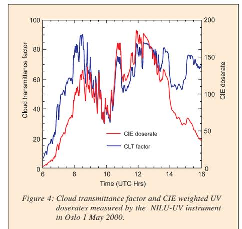
Figure 4: Cloud transmittance factor and CIE weighted UV dose rates measured by the NILU-UV instrument in Oslo 1 May 2000.
